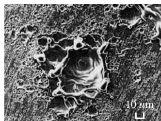
Photo 1 SEM image of crater by one pulsed spark discharge
